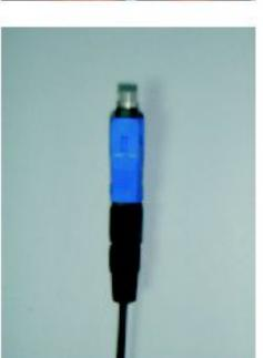
Turn the protrusion of housing toward the bottom and unite it to body. Completion.
