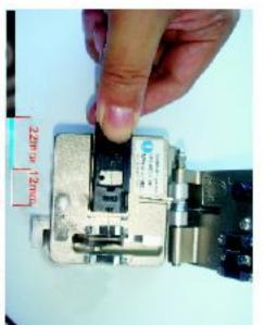
Cut off the fiber at the length of 12mm using optical fiber cleaver.
