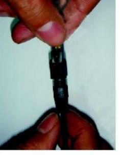
Take the boot cover down, connect the screw cap with boot by turning it and make the coating & strength member (yarn)fix.
