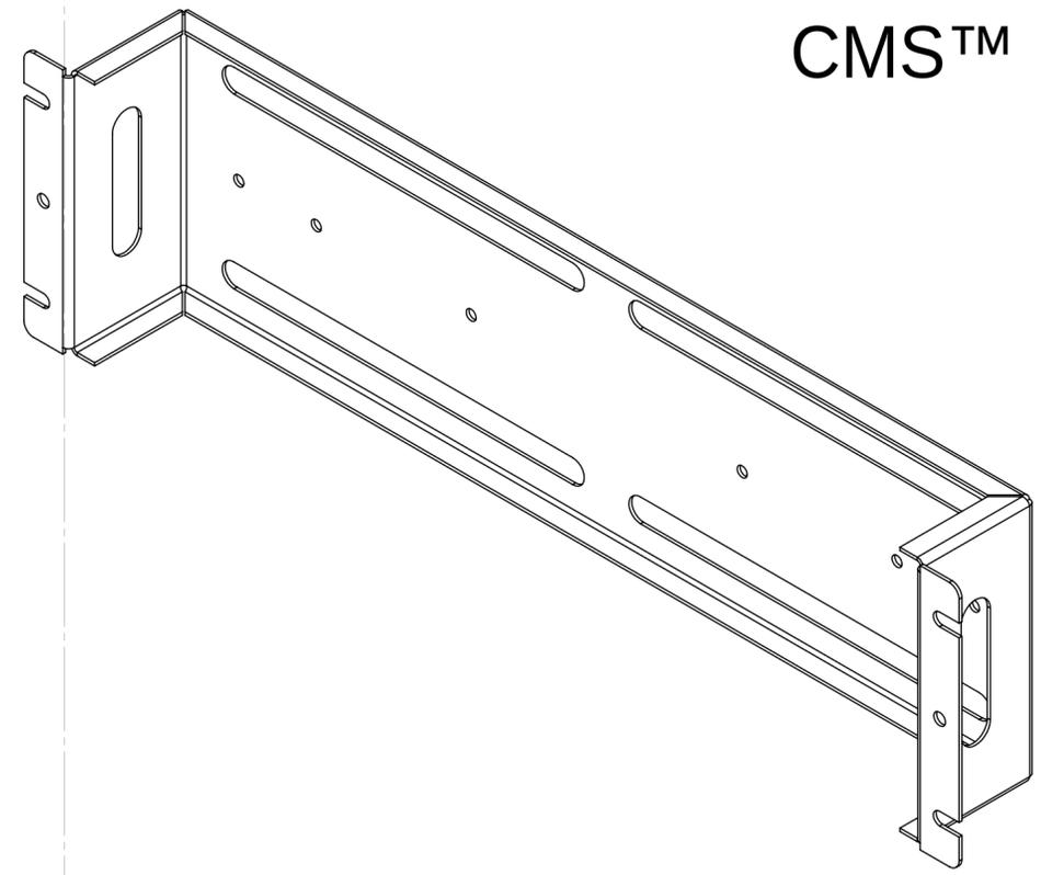
Electrical distribution panel 19" 3U with DIN rail is designed for circuit breakers, RCDs, differential circuit breakers, power sockets and other devices mounted on a DIN rail, mounted inside server cabinets or racks. The panel is made of steel, powder-coated. The panel has a capacity up to 24 circuit breakers up to 17.5mm wide. The panel design consists of two parts, the base and the front part. The base has a pre-installed galvanized DIN rail.
