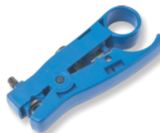
▶ KD-T7501A Coaxial stripper • With 2 Blades Strip cable for RG174/58/59/62/6/3C/4C/5C (OD2.6-8.0MM)
