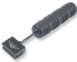
▶ KD-T2026 110 type punch down tool • For use on Lan and Telecom,seating 4 or 5 pairs UTP (24awg)at a time • Suitable for both 110 type cable side and cross-connect side terminals blocks
