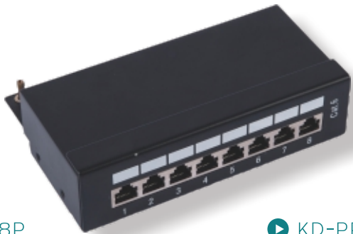
▶ KD-PP28-STP-C6-8P 10" 1U Desktop STP CAT6 8 Ports Krone&110 Dual IDC
