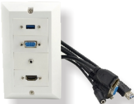
▶ KD-FP167 Multimedia Face Plate. • HDMI+VGA+USB+3.5mm Stereo Ports • UK Type • Length:20cm • Size:86X146mm
