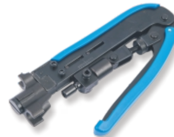
▶ KD-T548G201 Compression Tool • For crimping RG59,RG6 and RG11 for F/BNC/RCA type compression connectors • Can adjust the distance
