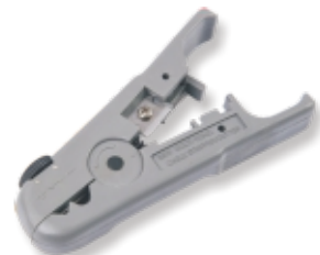
► KD-T501B cutter&stripper • For cutting or stripping UTP/STP or flat cable from 3.2mm-9mm • With adjustable knob for fitting different cable sizes
