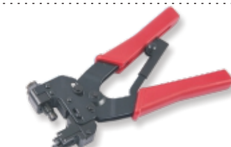
► KD-TH5081B Crimping Tool • For crimping F,BNC,RCA,right angled and keystone module compression connectors • With adjustment for crimping different length of connectors • With double color handle • With ratchet
