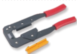
► KD-T214 IDC-TYPE Crimping Tool • For crimping IDC-type of connectors on ribbon cable • For crimping from height 6mm, distance to 275mm(max.55mm width)
