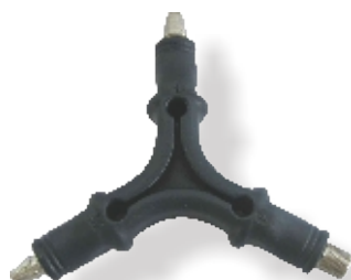
▶ KD-T224D Pin-Extractor 3 in 1 Tool one end to enlarge space between shield and insulation for RG59, another for RG6, the other end lock F connector into tool socket and twist it onto a stripped cable end
