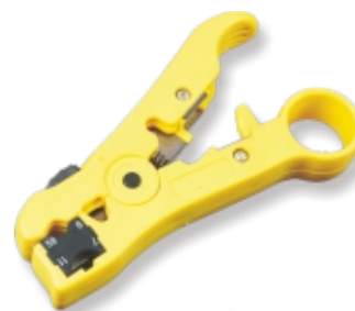
▶ KD-T352 Cable stripper • Adjustable stripping blade for different insulation thickness,prevents damage of shielding and conductor • The cassette can be reversed to change different coaxial cable • Strips UTP and STP cable,RG59/6/11/7 coaxial cable,flat telephone cable • With cable cutter
