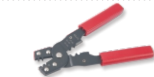
► KD-T202B Terminal Crimping Tool • For computer pins & sockets D-Sub 26-28 AWG wire • For butt-insulated connectors, 22-26 AWG wire • For telephone piercing spade lugs, 22-26 AWG wire • For open barrel connectors,20-22 AWG wire • For open barrel connectors,14-18 AWG wire • For non-insulated terminals,10-14,16-18 and 20-22 AWG wire
