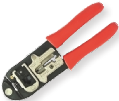
▶ KD-T3688 Crimping Tool • For Crimping 8P8C Plug • For Stripping Round Cable • For Cutting Cable
