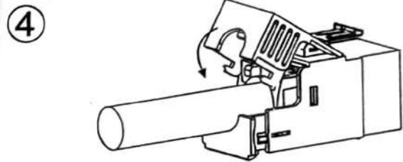
Press down the upper cover and push the wire cap to clamp the wire in place.
