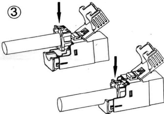
Place the network cable cap on the card from top to bottom, all the way down.
