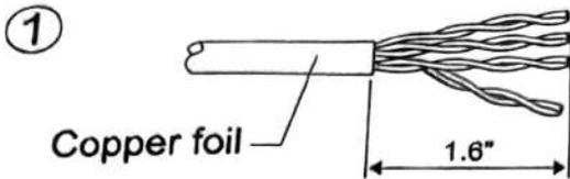
Strip off 1.6 inch of a cable jacket and fold braid back over it. Cut off aluminum foil for each pair, and use a supplied copper foil shield surrounding a cable.
