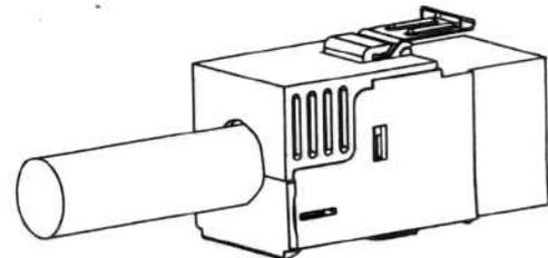
After pressing the upper cover to the bottom, push on the safety card to secure the top cover. By operating in reverse order, modules can be opened.
